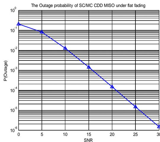
Fig. 2. The Outage probability of SC/MC CDD MISO under flat fading with three transmit antennas and  $R = 2$  b/s/Hz.
